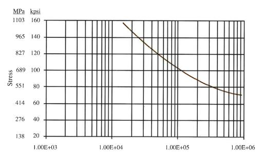
Number of Cycles to Failure Zero-to-Torsion Fatigue Elgiloy® Wire
